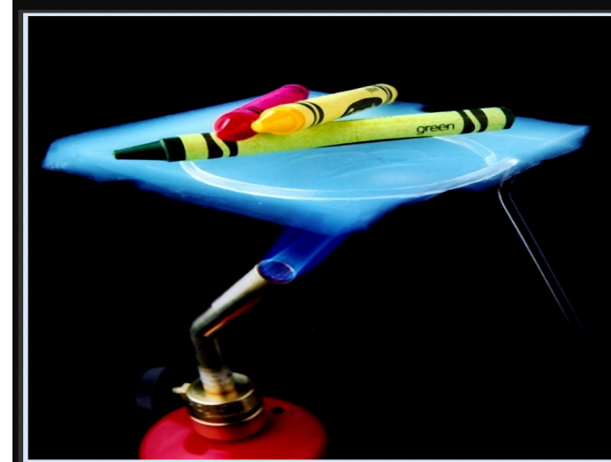
Silica aerogel tile insulating crayons from the heat of a blow torch
