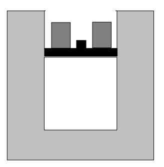
At time **C** we stop adding lead weights to the container and the piston stops moving. The piston is now at exactly the same position it was at time **A**.
