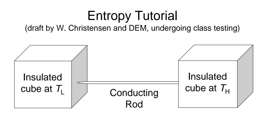
• Consider slow heat transfer process between two thermal reservoirs (insulated metal cubes connected by thin metal pipe)
