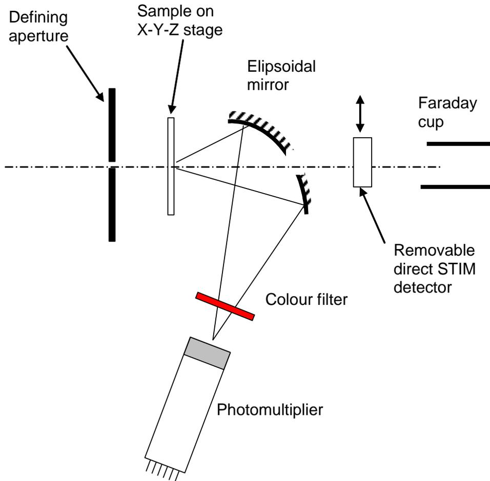
Fig. 4 Schematic illustration of set-up for MeV ion beam fluorescence imaging using the Jyväskylä PPAL system.
