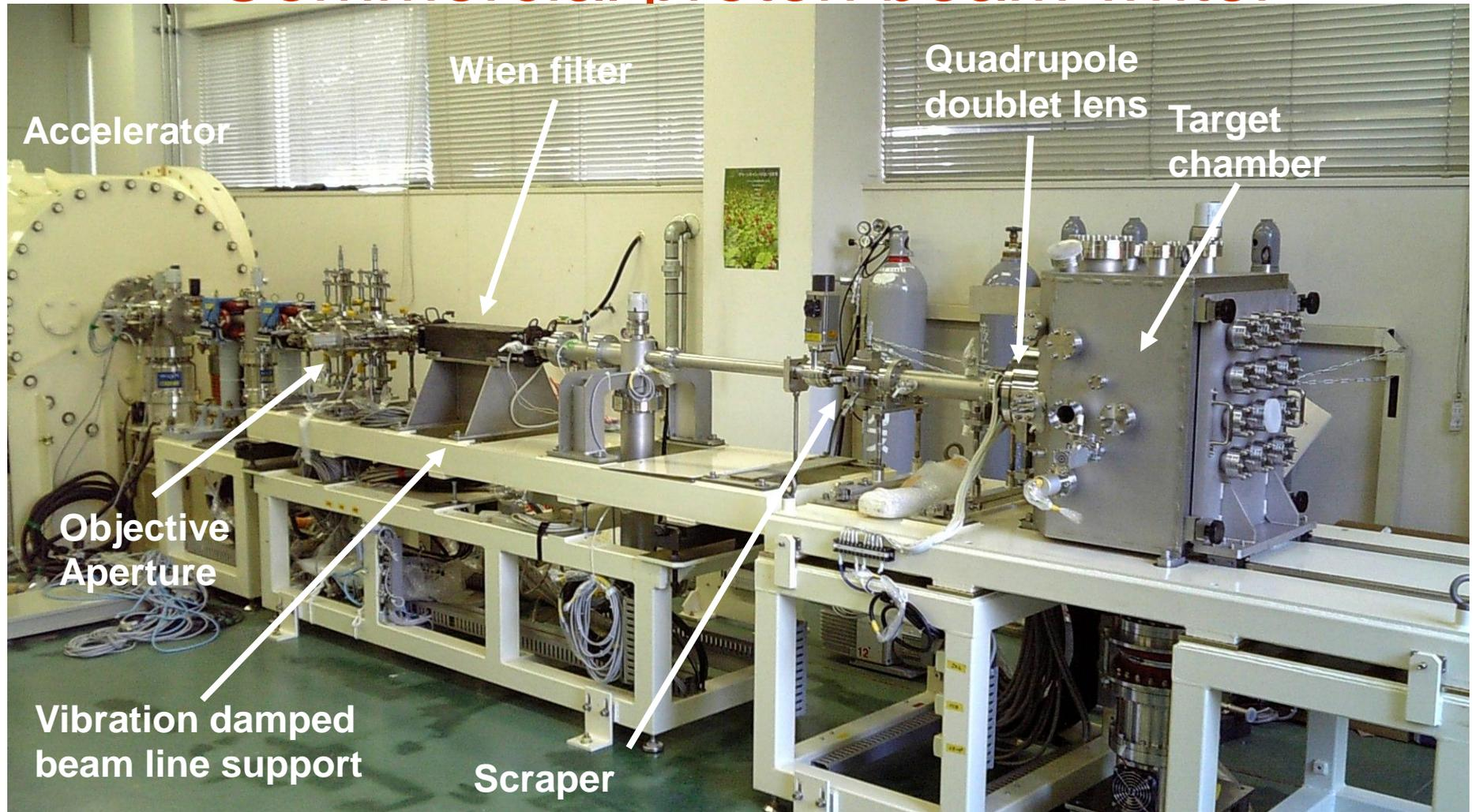
A commercial proton beam writing accelerator at the Center for Flexible Micromachining, Shibara Institute of Technology, Japan (S. Sangyuenyongpipat, H. J. Whitlow, S. T. Nakagawa and E. Yoshida, Proc CAARI 2008, American Institute of Physics, In press)
