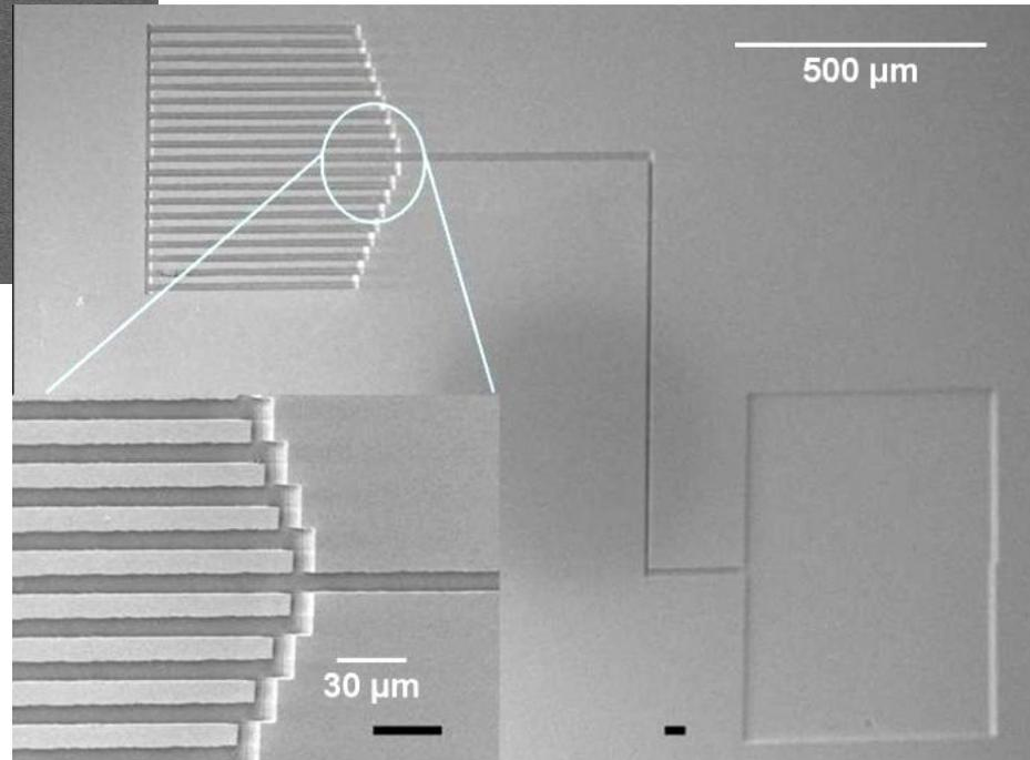
Prototype microfluidics structure comprising reservoir, capillary and micro pump. The PMMA structure is 12 μm thick and the channel width is 10 μm. (Liping Wang, Leona Gilbert and Harry J. Whitlow, University of Jyväskylä, unpublished results.)
